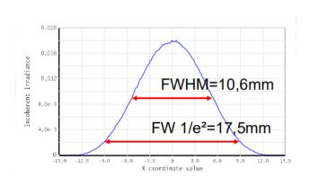
Spatial Distribution Pattern (Left) and Short Axis Spatial Output Profile (Right), 0.2 meters away from Diffuser
