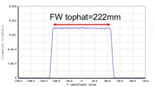
Spatial Distribution Pattern (Left) and Long Axis Spatial Output Profile (Right), 0.2 meter away from Diffuser
