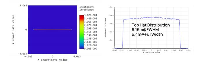
Spatial Distribution Pattern (Left) and Spatial Output Profile (Right), 3 meters away from Diffuser (6) Simulation based on DPSSL@1064nm, the original divergences of lasing diodes are FA@0.172deg and SA@1.335deg
