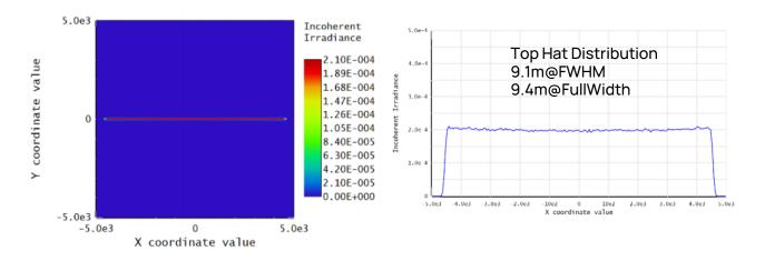
Spatial Distribution Pattern (Left) and Spatial Output Profile (Right), 3 meters away from Diffuser (6) Simulation based on DPSSL@1064nm, the original divergences of lasing diodes are FA@0.172deg and SA@1.335deg
